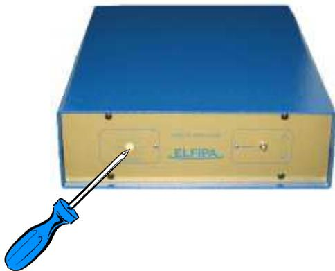
A. Phonopull connection to LAPORTE target release machine and use of the machine power supply for the Phonopull supply at 12 Vcc. This connection let remove the 220 Vac power outlet of the Phonopull.
