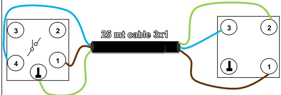
B. Phonopull connection to be used in those machines, which have a release button. This connection requires a 220 Vac socket for the Phonopull power supply.
