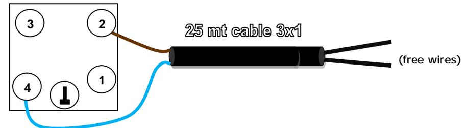
C. Phonopull connection to MATTARELLI target release machine and use of the machine power supply as a 24 Vcc power supply for the Phonopull. This connection let remove the 220 Vac power socket for the Phonopull power supply.
