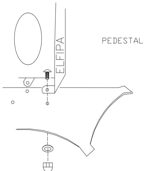
If the product is provided with the pedestal not assembled, fix it as in the picture, using the screws that are given in endowment.
