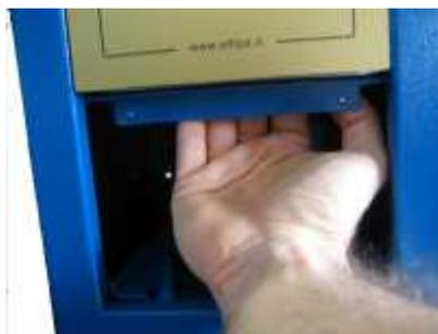
4. - Now flip the panel holding it with his hand. after closing the panel and lift up the latch and tighten the screws. See Fig.
