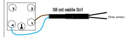
C. Phonopull connection to MATTARELLI target release machine and use of the machine power supply as a 24 Vcc power supply for the Phonopull. This connection let remove the 220 Vac power socket for the Phonupll power supply.
