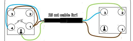
B. Phonopull connection to be used in those machines, which have a release button. This connection requires a 220 Vac socket for the Phonopull power supply.
