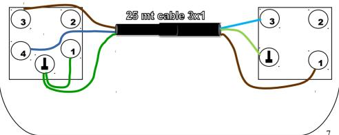
D. Phonopull connection to ELFIPA target release machine and use of the machine power supply as a 12/24 Vcc power supply for the Phonopull. This connection let remove the 220 Vac power socket for the Phonupll power supply.
