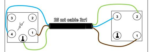
B. <u>Phonopull connection to be used in those machines, which have a release</u> <u>button. This connection requires a 220 Vac socket for the Phonopull power</u> <u>supply.</u>
