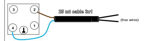
C. <u>Phonopull connection to MATTARELLI target release machine and use of</u> <u>the machine power supply as a 24 Vcc power supply for the Phonopull.</u> <u>This connection let remove the 220 Vac power socket for the Phonupll</u> <u>power supply.</u>
