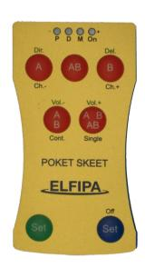
after the last calls the device turns off automatically if it's 'Single' or it's continued 'Cont.' until the push button BLUE 'Off'; the device will still turn off if there is no call after 3 minutes of inactivity.
