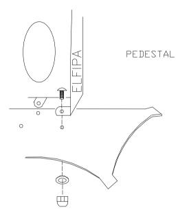
If the product is provided with the pedestal not assembled, fix it as in the picture, using the screws that are given in endowment.
