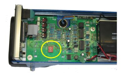
3- the jumper circled in red with the inscription SELECT is used to set the transmission mode. With the jumper connected equipment is turned on after each call, vice versa with jumper removed after a call turn off.
